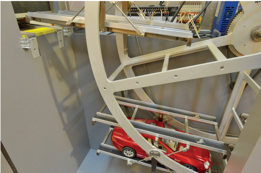
Fig. 4. Rotary car park – model, car view on the platform
